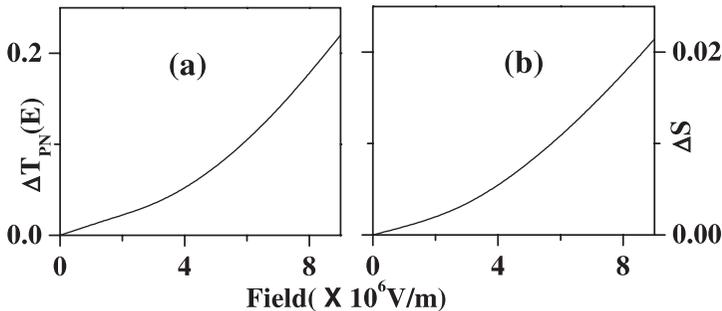
Fig. 3 – (a) Calculated variation of  $\Delta T_{PN}$  as a function of electric field. (b) Calculated variation of  $\Delta S$  in the nematic phase at  $T_{NI} - 0.1^\circ$  as a function of field.
