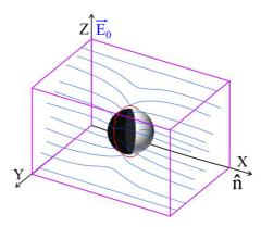
FIG. 2. Quadrupolar director field surrounding a Janus particle. The applied electric field  $\mathbf{E}$  is transverse to the director. The red circle denotes the Saturn-ring defect. The black hemisphere represents metal.
