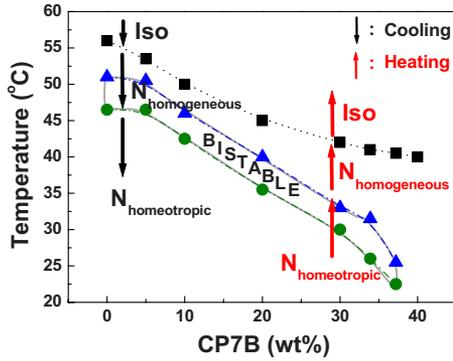
FIG. 4. (Color online) Transition temperatures as a function of the concentration of CP7B in the CCN-47/CP7B binary mixture system. Iso and N stand for isotropic and nematic phases, respectively. The area between triangular and circular symbols represents bistable regime, i.e., both planar and homeotropic alignments are stable.
